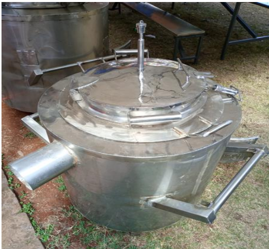
An example of an energy saving commercial pressure cooker that can use both firewood and LPG. This is suitable for schools and will cut cost and reduce impact on human health and the environment.
