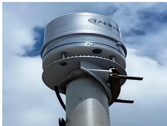
‘All in one’ sensor suite for the automatic weather
